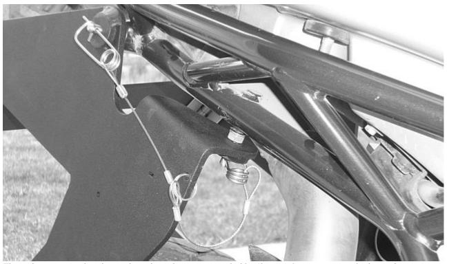
The safety pins in the above photo have been superseded by 'bow tie' cotter pins, which are far easier to use, very secure, and more robust.
