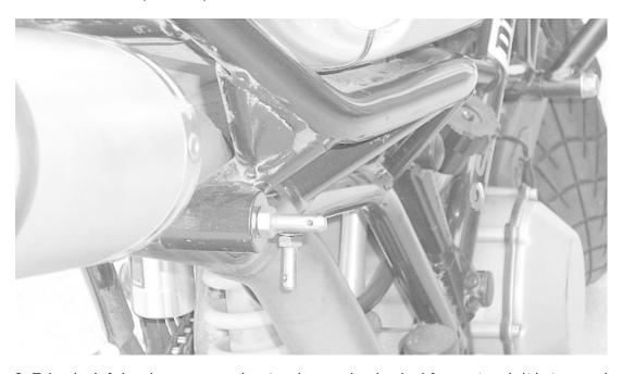
3. Take the left hand case mount (leaving the crossbar latched for now) and slide it onto the rear stud first, then hinge it up so the forward mount stud goes through the hole in the case mount. Note that there are two 'bow tie' cotter pins on different-length lanyards; put the longer one through the rear mount, and the shorter through the front. Repeat the same process for the right side.
