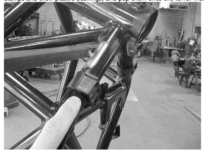
4. Install the front mount plate and secure it with the M8 locknuts. Do not tighten the nuts all the way at this point, as you will need to adjust the mount location prior to applying final torque.
